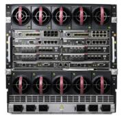
Figure 1-2 is an illustration showing the location of the device bays, power supply bays, and the Insight Display at the front of the HP BladeSystem c7000 enclosure.
